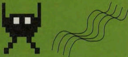
■ Spot the difference. The invader is a bitmap image made of pixels, while the wavy lines are theoretical, being smooth from any distance.
