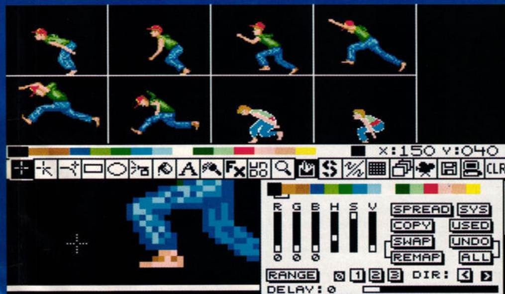
● Using either the Control Panel Accessory - CONTROL.ACC (above) or sliders such as those in the art package DeluxePaint (below) you can alter the levels of red, green or blue light to create the shade you want.
