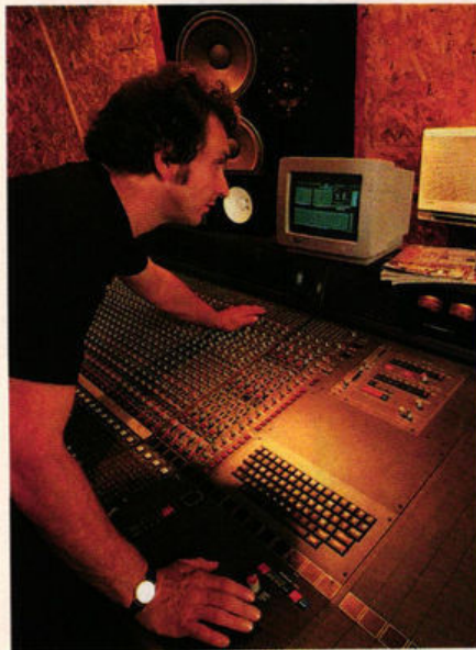
■ Big George at the Mozart recording desk. The non-standard keyboard just in front of his right hand disguises the fact that this £70,000 piece of hardware is built around a Mega 4 ST: his right hand rests on the built-in tracker mouse that operates the ST-based Supertrue Automation software showing on the mono monitor
