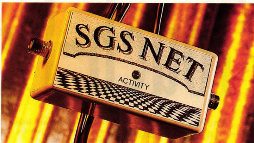
■ SGS Net uses the MIDI ports to network the ST, providing a cheap and effective solution to the problems of peripheral and program sharing
